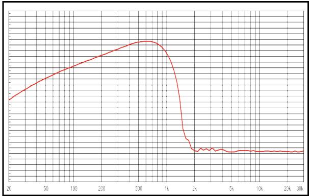
FIGURE 24. Frequency Response - Preset 2 (300Hz to 900Hz)
