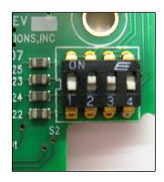
Switch 1 - OFF Switch 2 - ON Switch 3 - ON Switch 4 - OFF
