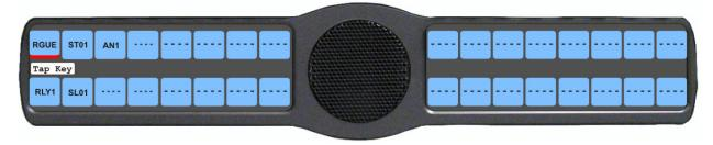
**6.** Tap **down** on any keypanel key you want to assign the exclusive key option. *The selected keys return to the unassigned state (light blue color).*
