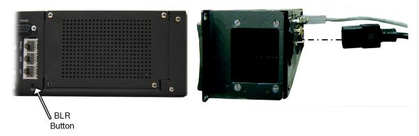
**4.** While the BLR button is pressed, connect the **power cord** to the keypanel. *KP 32 CLD - Boot Loader Waiting for download... appears in the display window.*
