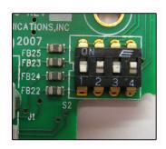
Switch 1 - OFF Switch 2 - ON Switch 3 - OFF Switch 4 - ON
