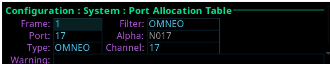
**NOTE:** To move from field to field, rotate the right encoder knob. To scroll the screen up and down, rotate the left encoder knob. To modify a field click the right encoder knob. To exit a screen click the left encoder knob.
