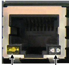
**Left LED.** The left LED is yellow and indicates a network link is established. It flashes on/off whenever there is network activity.
