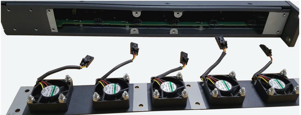
**IMPORTANT:** Care must be taken to depress the locking feature (1) on each harness connector before disengaging. Wire and/or receptacle damage can occur if not properly removed.
