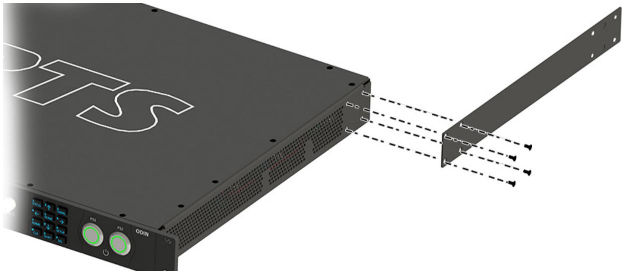
**IMPORTANT:** Alternately, attaching the rear side brackets before putting the ODIN frame in the rack is possible. The frame may need to be slightly tilted for the rear side bracket to clear the back of the rack before securing it to the rack.
