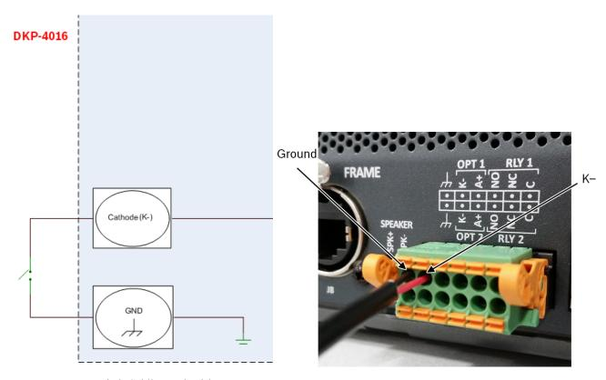
FIGURE 4. Footswitch Cabling and Wiring
