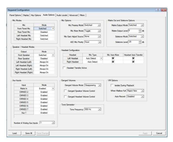
FIGURE 54. Keypanel Configuration – Audio Options
