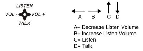
FIGURE 7. Key Function Position Explanation
