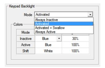
FIGURE 37. Display Page – Keypad Backlight Group Box
