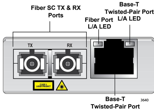
Figure 10. AT-MMC2000/200 Series *nn*/SC Front Panel
