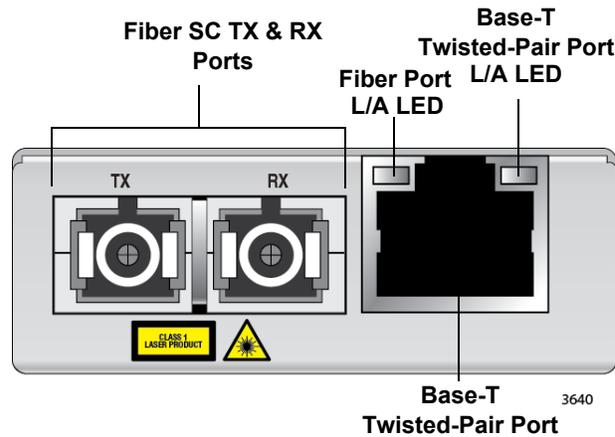
Figure 10. AT-MMC2000/200 Series *nn*/SC Front Panel
