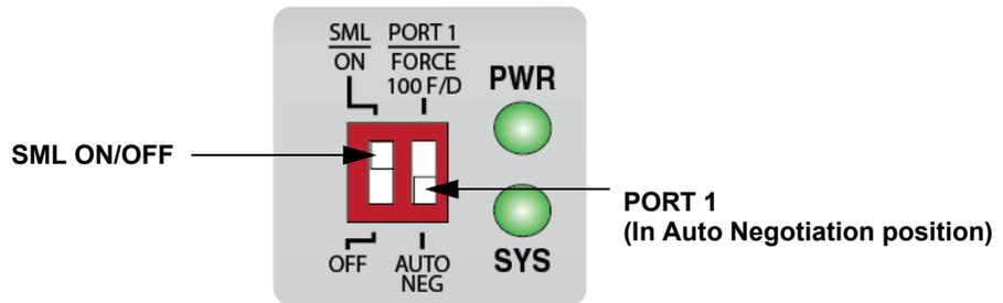
Figure 9. AT-MMC2000/200 Series Converter Rear Panel DIP Switches
