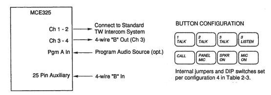
Figure 1.6 Standard two-channel, four wire configuration.
