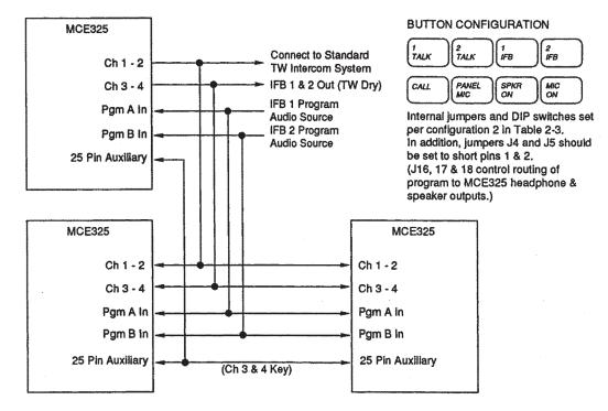
**Figure 1.8** Multiple interconnected stations using one four-wire intercom channel and two two-wire channels for IFB's.
