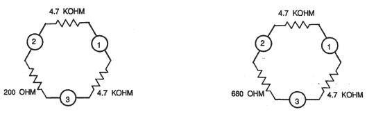
When four-wire outputs are used, termination resistors must be installed for proper operation. The output amplifiers are current sources, and the output level is determined by the terminating
