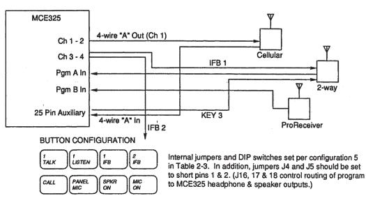
Figure 1.11 MCE325 button configurations.
