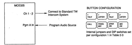
Figure 1.3 Standard four-channel, two-wire configuration.
